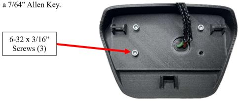
4. Attach the Plastic P-Clamp around the Coiled Cable, screw the P-Clamp the bottom right Switch Panel hole using the 6-32 x 5/16" Screw (1) provided and a 7/64" Allen Key. Plug the Coiled Cable to the Switch Panel and route the cables as seen below.
