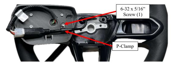
5. Tuck cables underneath the steering wheel trim and attach the plastic cap to the steering wheel. Ensure the cables are not pinched and all three mounting tables are clipped in. To remove the plastic cap from the steering wheel, pinch the top and bottom walls of the mount and gently pop it off. Connect the Coiled Cable to the system's Communications Cable. Zip-tie the cables under the dash so
