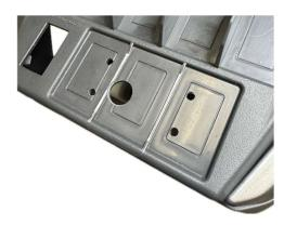
6. Using a pair of cutters/clippers, clip off the guide holes from the Steering Wheel Mount. Make the cut as flush as possible to ensure the Switch Panel fits. Discard the guide holes.
