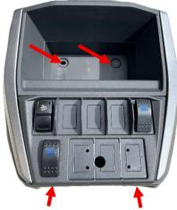
2. Using diagonal cutters, carefully cut off the 3 fins separating the bottom 3 rocker switch cutouts. Use a razor blade to make the cuts flush to the dash.
