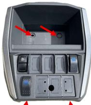
2. Remove the rocker switches and carefully cut the dashed line. Use a Dremel or a cutting tool.
