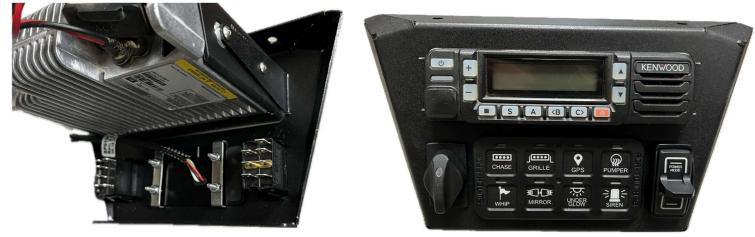
4. Place the mount onto the dash, hold it flush and mark the 2 top holes and 2 bottom holes. Using the 1/4" Drill Bit, drill the 4 holes into the dash.
